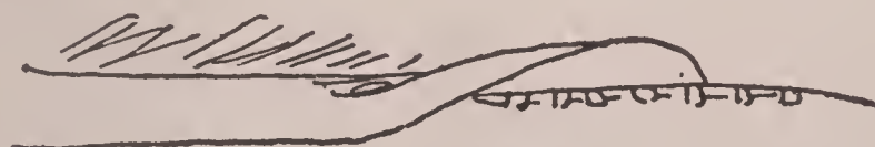
Fig. (7) The tape rolled onto the wrong side
